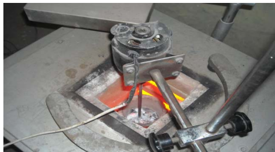
Fig. 2: stir casting setup
